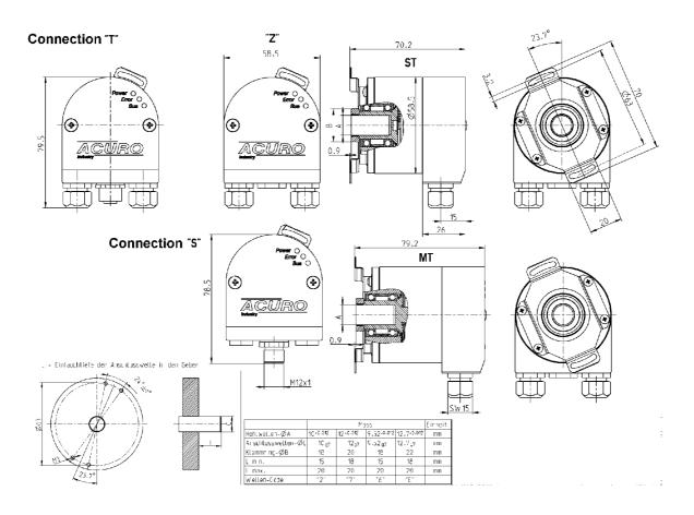
The cable screw connections require cable diameters in a range from: 7.0...7.4 mm.
