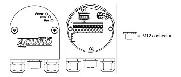
$\Rightarrow$  Loosen the screws and draw off the bus terminal box from the encoder.
