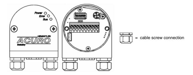
$\Rightarrow$  Loosen the screws and draw off the bus terminal box from the encoder.
