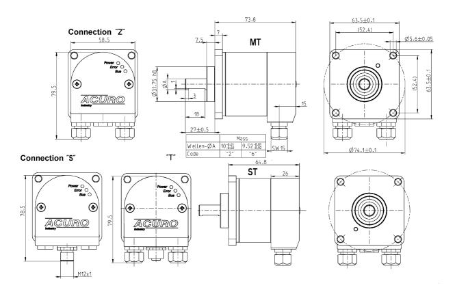
• The cable screw connections require cable diameters in a range from: 7.0...7.4 mm.
