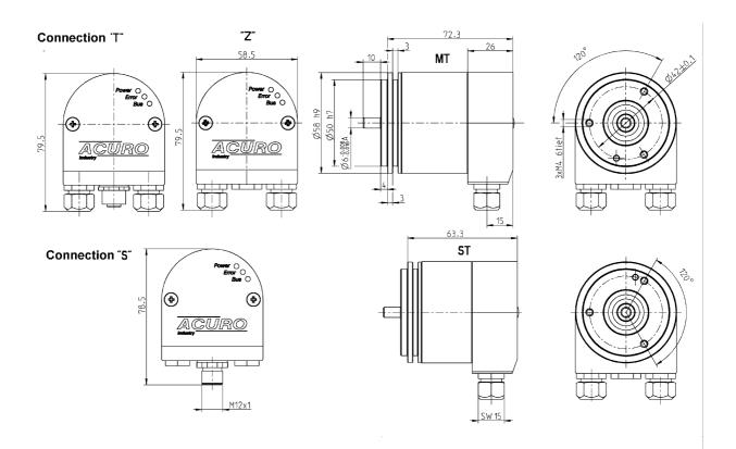
The cable screw connections require cable diameters in a range from: 7.0...7.4 mm.
