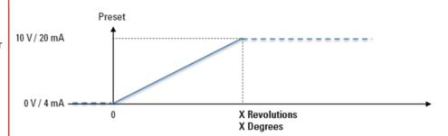
Default Setting: Output signal rotation cw (clockwise) with a view to the shaft.
