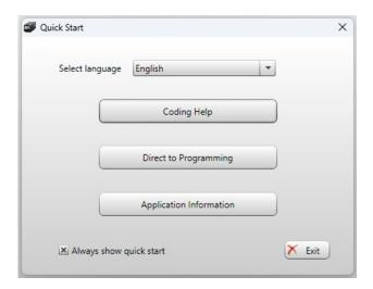
10. Selecting "Application Information" opens window with Settings of the product for most common applications. After choosing "Select" the specific settings are used and the program will start. These settings can then be modified by the user directly in the Program.
