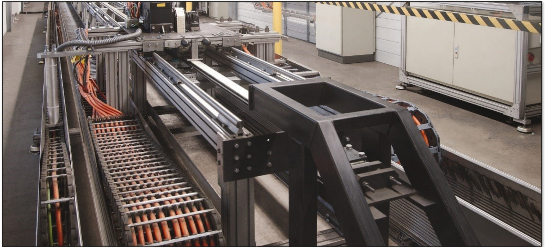
Drag chain test systems at Helukabel's research and development center.
